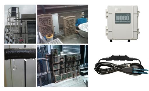
Figure 20. Irrigation system components. Figure 21. Hobo U30 Monitoring System. Figure 22. ECHO EC-5 Soil Moisture Sensor.
